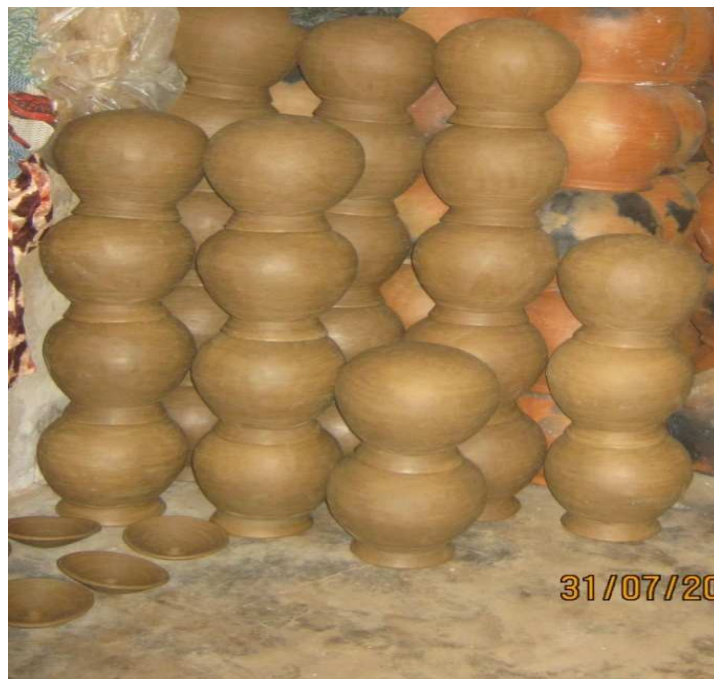
Plate 8. Pots are then left to dry till they are ready for firing
