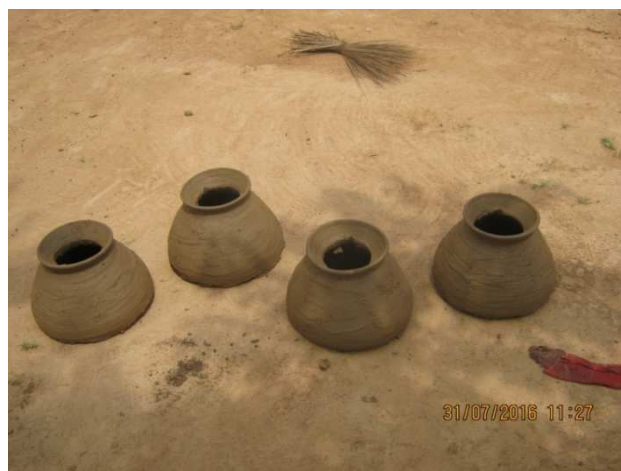
Plate 5. Formed rough blended body
