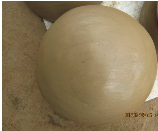
Plate 7. Smoothened round base formed
