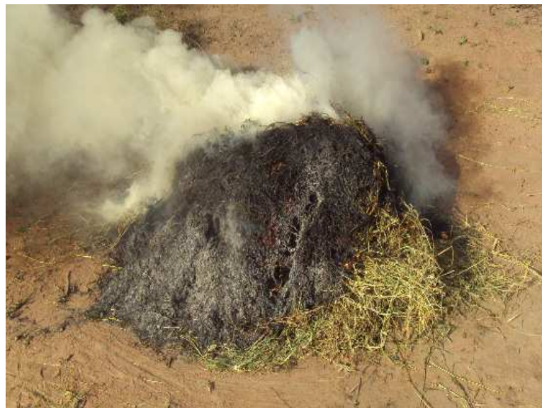
Plate 10. Dried pots are then fired in the open
